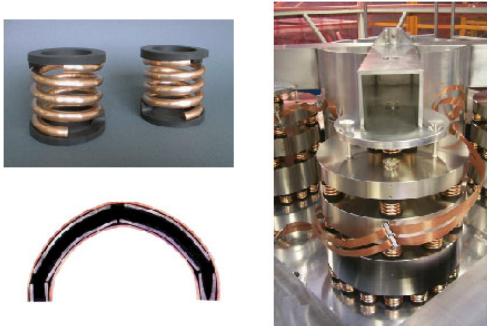
Figure 4: Four-layer seismic stack (right), with inverted optical table resting upon top layer of springs; a pair of springs (upper left), ~7.5 cm high prior to compression; spring coil cross section (lower left) shows internal damping material constrained between internal slug and outer spring wall.
